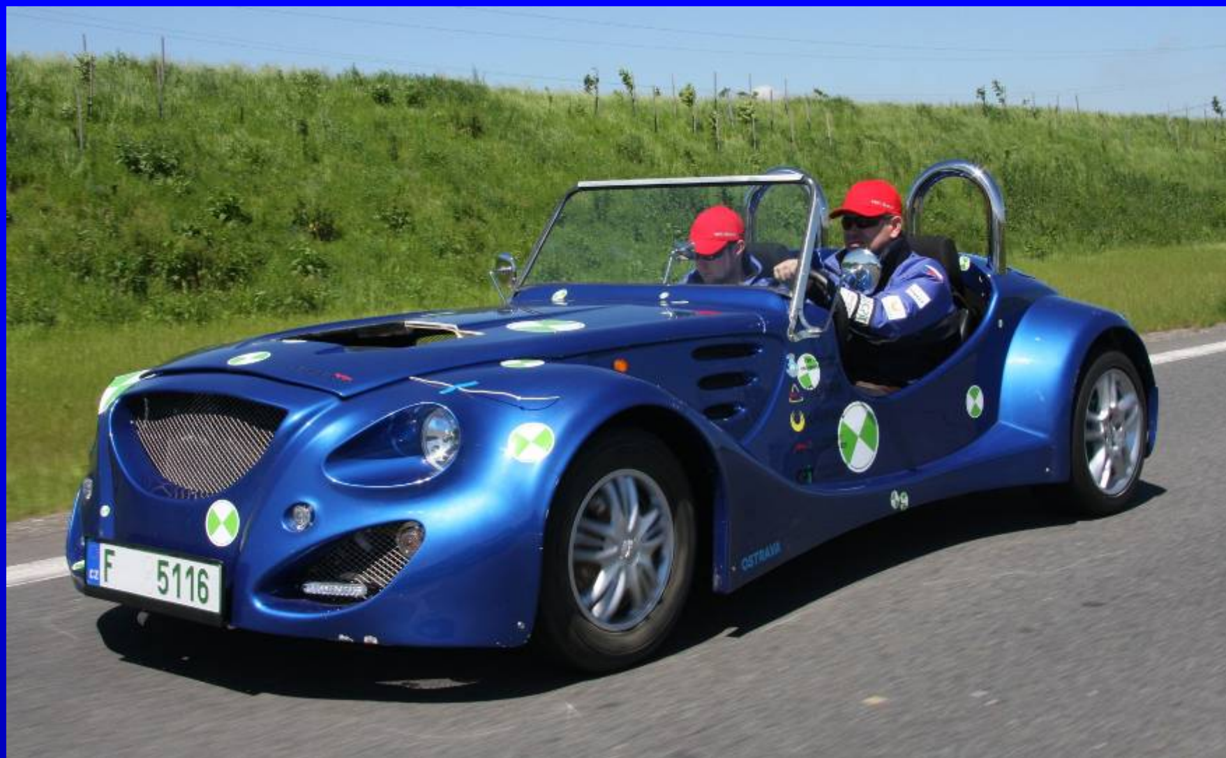
Obr.9. KAIPAN VoltAge K0 (2010-2013, 100km/1nabití/10kWh).
